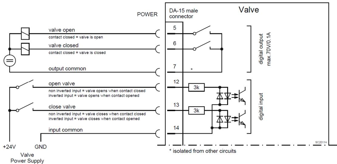
4.4.3.2 Power connector: Configuration with voltage source for digital inputs
