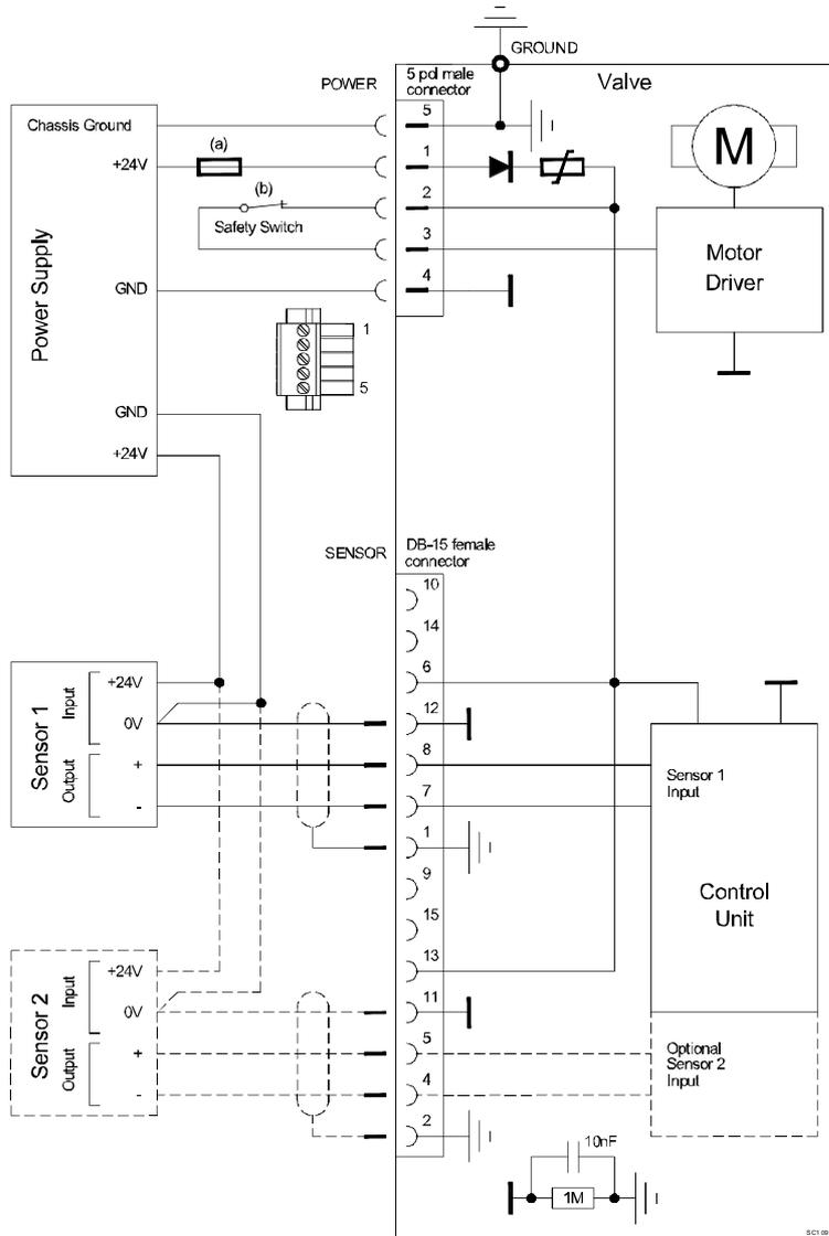
Pins 2 and 3 must be bridged for operation. An optional switch would allow for motor interlock to prevent valve from moving.
