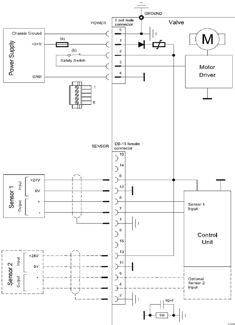
Pins 2 and 3 must be bridged for operation. An optional switch would allow for motor interlock to prevent valve from moving.
