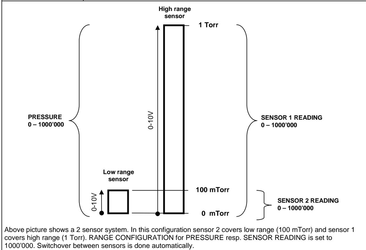
Above picture shows a 2 sensor system. In this configuration sensor 2 covers low range (100 mTorr) and sensor 1 covers high range (1 Torr). RANGE CONFIGURATION for PRESSURE resp. SENSOR READING is set to 1000'000. Switchover between sensors is done automatically.
