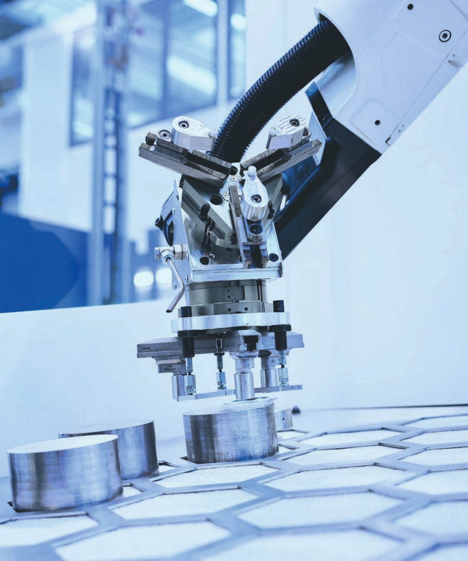
Fully automated Robot2Go system in the turning and milling area in Switzerland, enabling the efficient loading and unloading of raw materials and finished products
