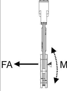
The diagram shows a vertical valve stem assembly. A solid arrow labeled 'FA' points horizontally to the left, representing an axial force. A dashed curved arrow labeled 'M' indicates a bending moment applied to the stem.
